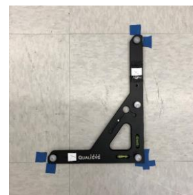
Put the L wand kit on the zero points of Vol. The long side will be the X axis.
